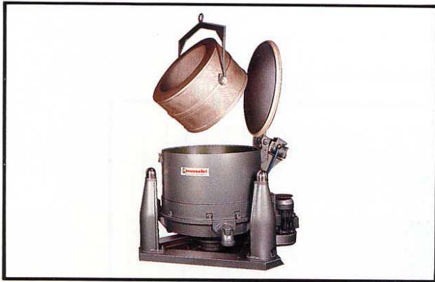
Centrifuge SC 70 KC to remove oil from swarf and components
