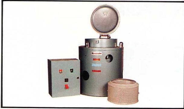
SA-KC : Centrifuge SA40 KC to remove oil from swarf and components
