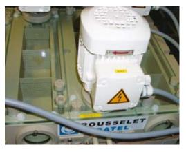
MD UX 2-1 : detail of a single stage with engine (mixer) and settler (static decantation area)
