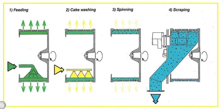
Figure 1: Horizontal Basket Filtration Cycle
