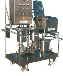
With peripheral equipment (storage containers for feeding solution, cake washing liquid and filtrate, and general control cabinet mounted on manual trolley with wheels).
