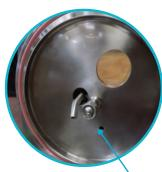
Neutral gas feeding piping allowing to work under flowing nitrogen.
