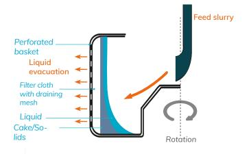
In this case the slurry can be fed into rotating basket.
